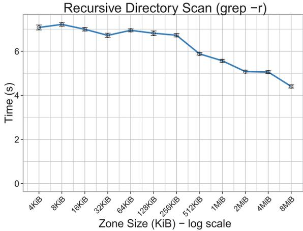
Fig. 5. Recursive scans of the Linux 3.11.10 source for “cpu\_to\_be64” with different BetrFS 0.2 zone sizes.
